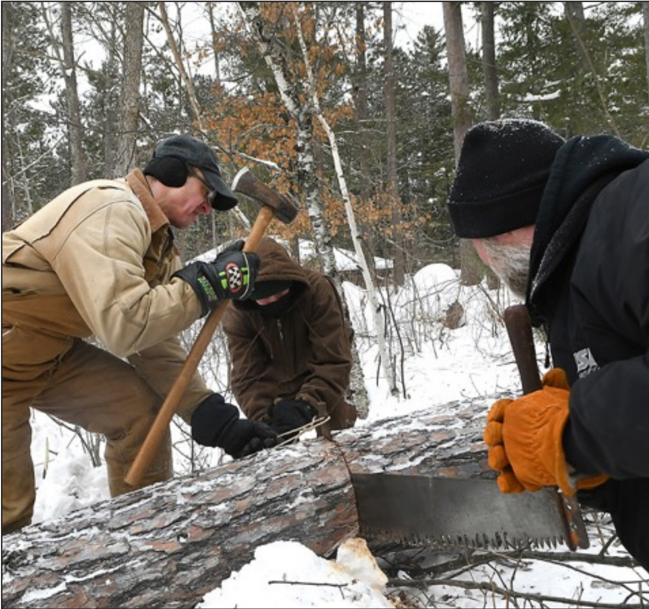
Fred Hemmerich, Zimmerman, Minn., drives a wedge into a cut, assisting Caleb Wright, Nevis, and Steve Skadsem, Detroit Lakes, as they use a double crosscut saw to cut sections out of freshly fallen tree.
